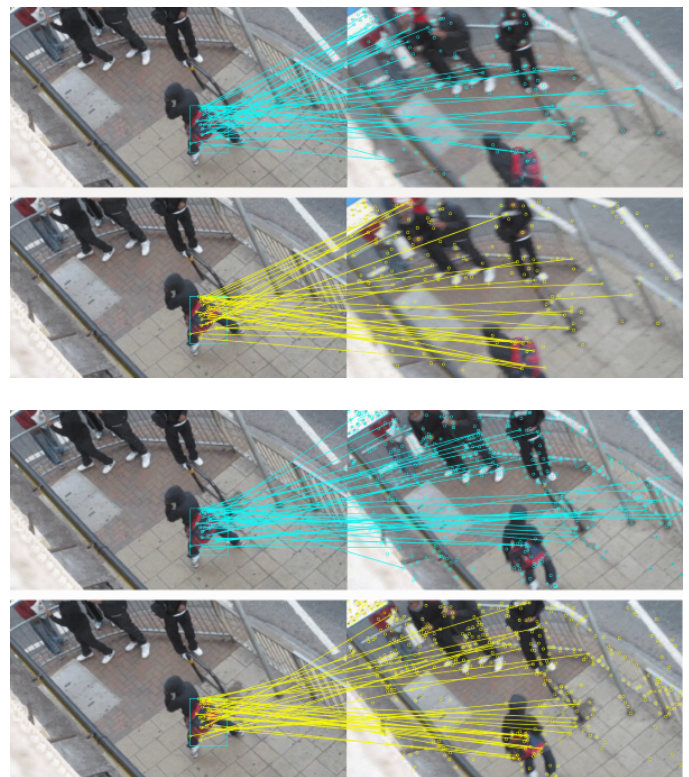
Fig. 6: Two examples of matching SURF features on a coloured bag from a query frame (left in each pair) to a subsequent video frame. Top, matches to a blurred image perform poorly using Approximate Nearest Neighbour (blue matches) and a significant increase in matches to the target bag using our method (yellow matches). Bottom demonstrates the significantly reduced number of false positive matches to the background using our method (yellow) compared with ANN matching (blue).
