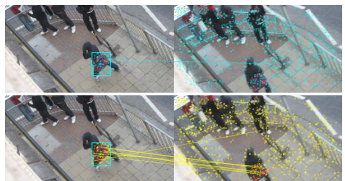
Fig. 7: Good matches – Equation (13) – are shown for SURF features (top row) and using our method (bottom row).
