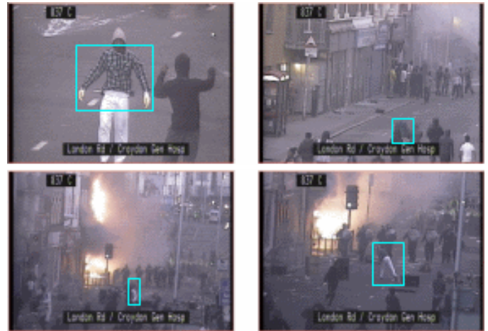
Fig. 1: Typical images from a single CCTV camera, with poor lighting and long range camera views. When a subject appears in the distance, the colour and texture definition is poor and inconsistent with frames when the subject is closer.
