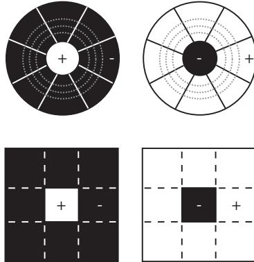
**Fig. 3.** Receptive Fields. The receptive fields of natural visual systems are circular and vary in size. This has been simplified to receptive fields with square zones of a fixed size of 3 by 3 pixels.
