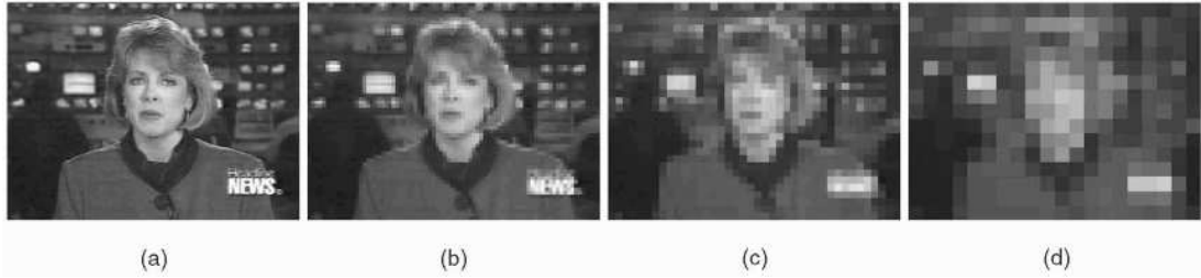
Figure 2.2: The multi-resolution hierarchy images created by averaging and sub-sampling, reproduced from Yang and Huang [97]. (a) Original image. (b) n=4 . (c) n=8 . (d) n=16 . From left to right, the figure shows the original image and lower resolution images in which the intensity of each pixel is replaced by the average intensity of n \times n pixels.
