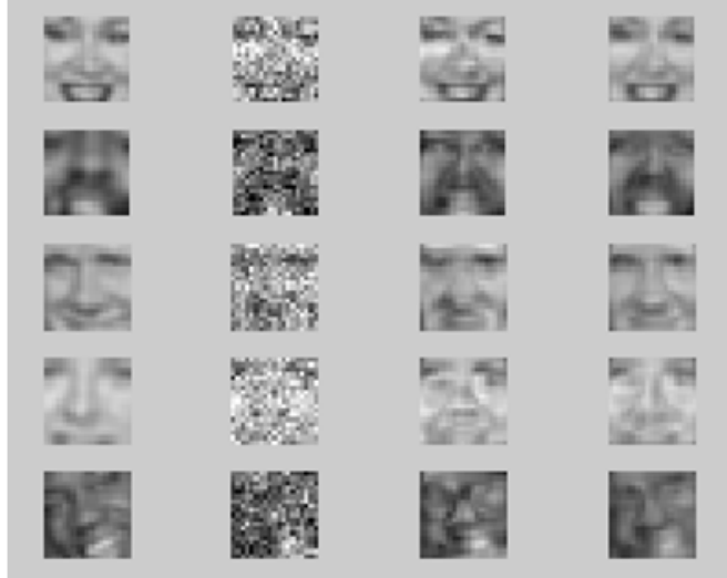
Figure 3.7: Re-construction of images under strong noises using PCA and ICA projections. From left to right, the images are the original images, images with strong noise, re-constructed images using PCA projection and images using ICA projection.
